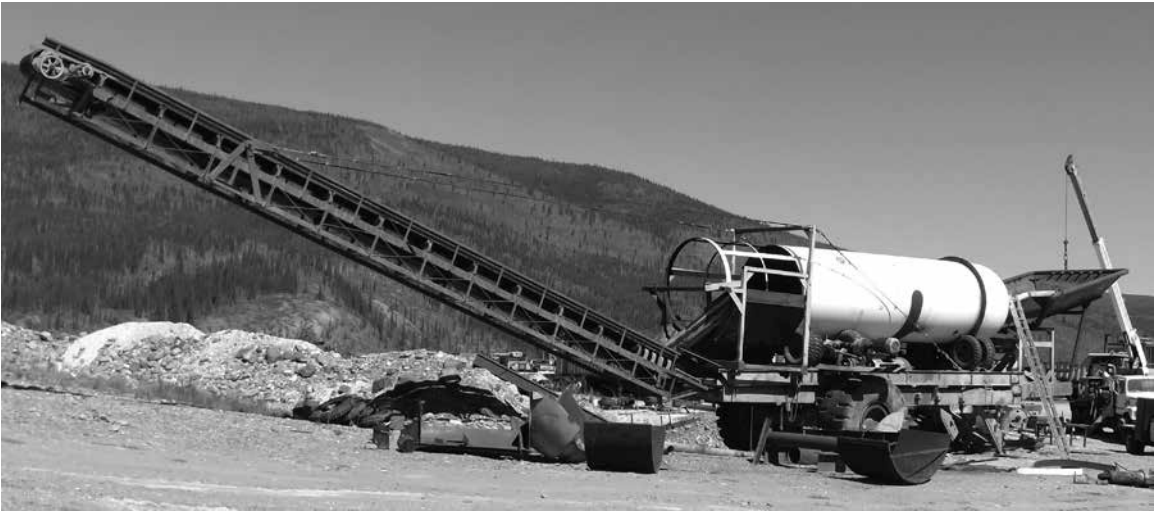
This trommel was mostly fabricated from re-used materials here in Dawson City. Josée Bonhomme is the owner and principal of a small local consultancy engaged in permitting for placer mines since 2003.
